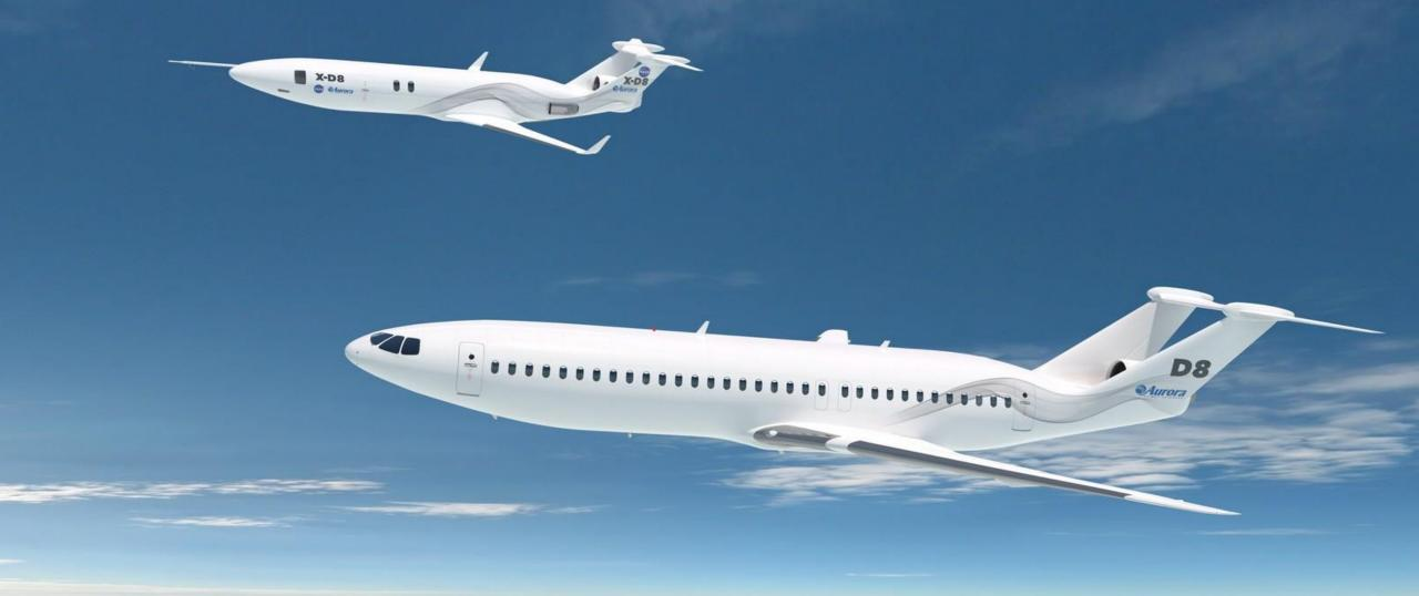
Aurora Flight Services (now being acquired by Boeing) is set to continue developing the subsonic D8 X-Plane (XD8). NASA has awarded the firm with a 12-month contract. The XD8 program aims to demonstrate key technologies of the D8 commercial aircraft concept. The aircraft could improve fuel, noise and operational efficiencies within the next decade, according to Aurora.
